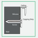
You may choose to fit the sheet tight to the ceiling (allow 3mm for expansion) and seal using the appropriate coloured silicone instead.
