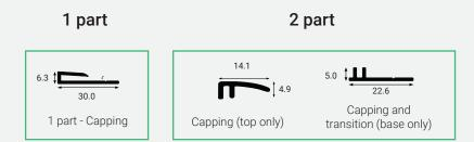
Capping profiles are used to create a watertight seal between the sheet and the ceiling/flooring.
