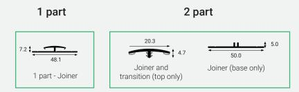
Joiner profiles are used to create a watertight seal between the sheet and the ceiling/flooring.
