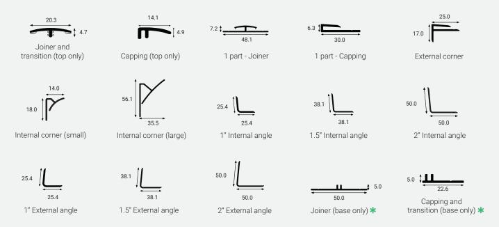
Lengths: 2440mm • 3050mm (Dimensions shown in mm)
